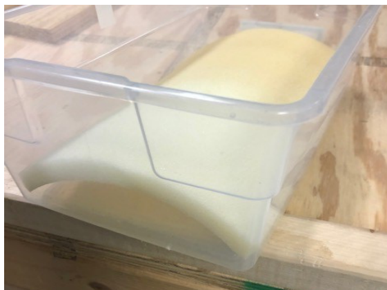
Over-sized 6.5” width of tub foam liner creates a soft arch in bottom of the tub.
