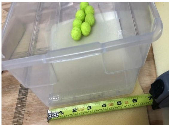
Over-sized 6.5” width of tub foam liner creates a soft arch in bottom of the tub.
